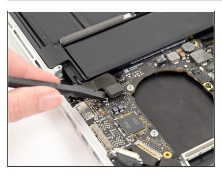
Pry the headphone jack cable connector up off its socket on the logic board.
