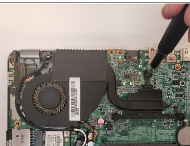
Remove the five Phillips #0 screws that are holding the fan down to the base.
