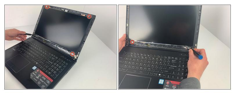
Remove the four 2 mm screws on the bottom and top corners of the screen using a Phillips #0 screwdriver.
