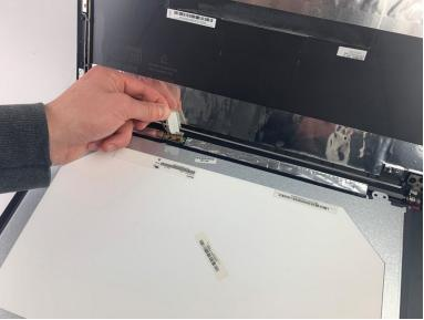
Remove the ribbon cable by pulling on the bar code tab.
