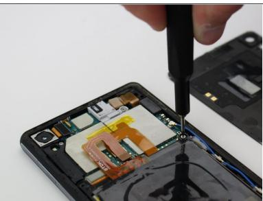
Use the Torx T5 screwdriver to remove the two 3.81mm screws from the corners of the battery.
