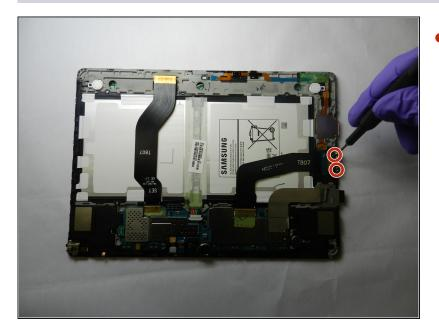
Using a Phillips #000 screwdriver, remove two screws on the ribbon cable bracket.
