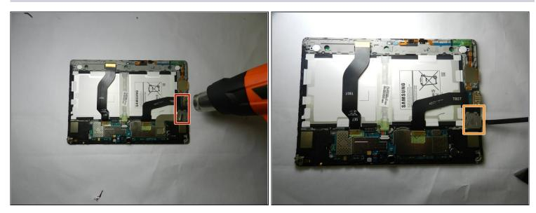
• Use a heat gun on the heat bracket and gently pry up the bracket.
