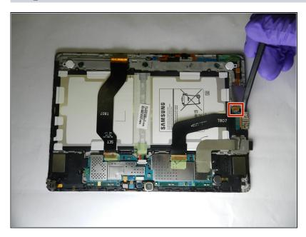
• Using a spudger, lift up the flex connector.
