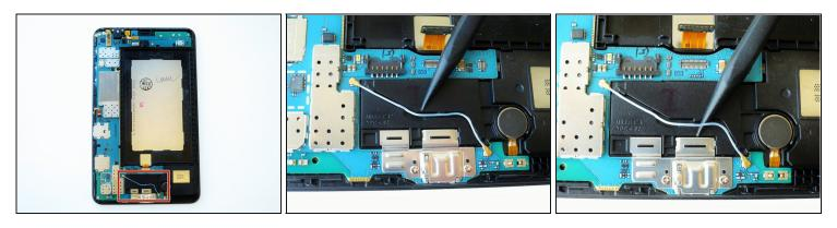
• Using the spudger gently wedge the blue wire out of its compartment.
