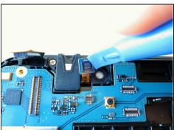
• Slightly apply pressure and move the blue plastic opening tool downwards to pop the gold square connector from its socket on the mother board.
