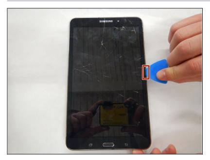
Insert an opening pick in between the display screen and the display frame.
