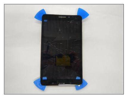
Wedge four of the opening picks in between the display screen and the device backing on all four corners.
