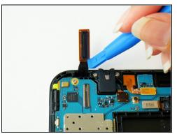
• Slightly apply pressure and move the blue plastic opening tool downwards to pop the gold rectangular connector from its socket on the mother board.
