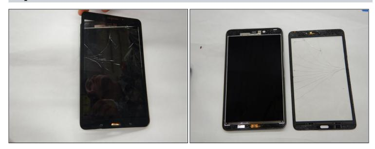
• Once the display is completely disconnected from the device gently remove it without touching the screen which lies underneath.
