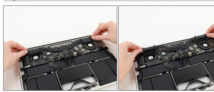
Lift and remove the heat sink up off the logic board assembly.
