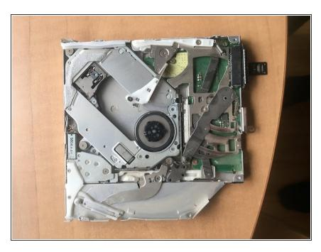
If I remember correctly, the aluminium and hinges held the cover on. With the aluminium off you can now enter deeper into the drive.
