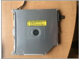
There is aluminium foil sticky tape that covers how the drive is split. You can see how the drive is split after having removed the tape. Now that you know how it is split you can probably make a nicer rip than me.
