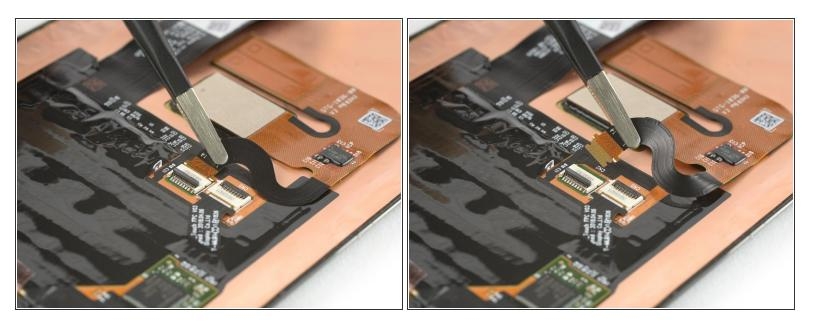
Use a pair of tweezers to carefully pull the flex cable of the fingerprint sensor out of the ZIF connector.
