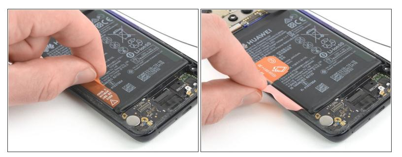
• Peel the orange adhesive strip labeled with a **2** off the battery. The orange adhesive tape will rip along a small perforated line.
