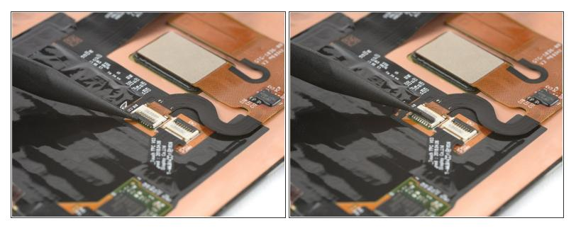
• Use the pointed end of a spudger to open the ZIF connector of the fingerprint sensor.
