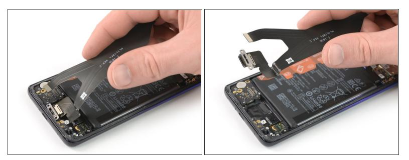
• Remove the main flex cable including the charging port by lifting it upwards and then pulling it in the direction of the motherboard.
