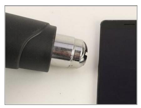
With caution to hot temperatures, glide a heat gun over the outer edges of the phone bezel to soften the adhesive securing the back panel to the phone.
