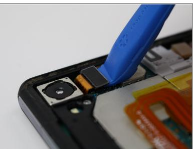
Using the plastic opening tool, carefully pry off the flex connector beside the camera housing.
