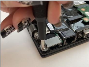
• Unscrew the single, 3.0 mm screw with a Phillips #1 screwdriver bit that holds the charging port housing into place.
