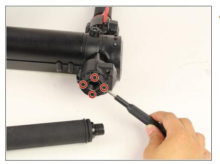
Remove four 2 mm Phillips #00 screws located on the acceleration throttle.
