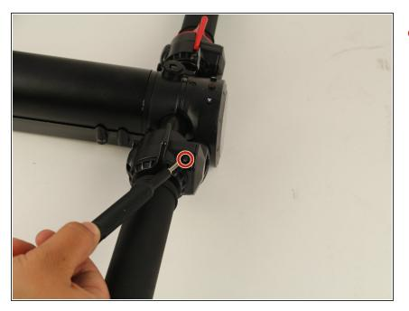
Remove one 4 mm Phillips #1 screw located directly above the acceleration lever.
