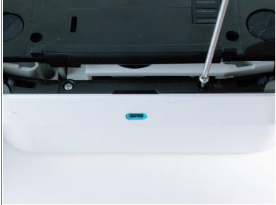
• Remove the two 22.0 mm screws on the bottom-front of the robot using a Phillips #1 screwdriver.
