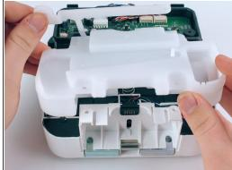
• Pull up on the L - shaped plastic piece and remove it from the tank assembly.
