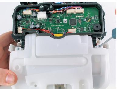
Use a Phillips #1 screwdriver to remove the two 9.7 mm screws on the tank.
