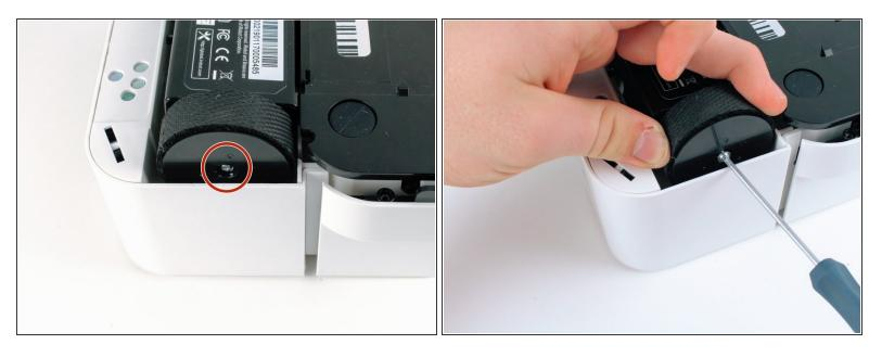
Remove the 11.55 mm screws in the middle of both wheels using the Phillips #1 screwdriver.
