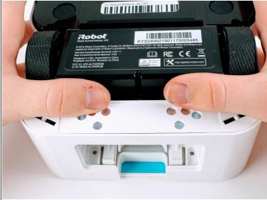
Using your thumbs, first push back the motor assembly, then push up.
