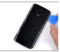
• Slide the pick along the right edge of the rear glass to separate the adhesive underneath.
