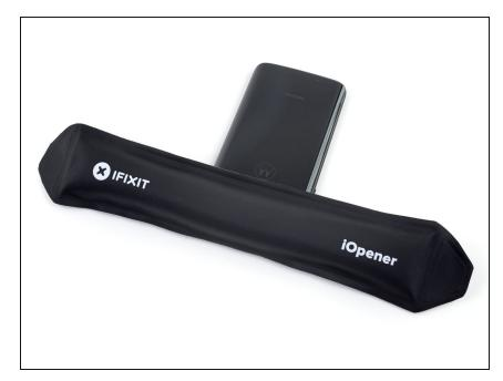
Heat the top edge of the back of the phone to soften the rear glass adhesive.
