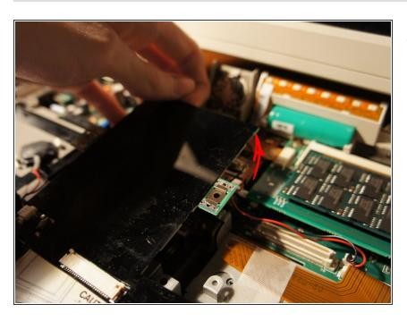
Carefully but firmly lift up the top part of the daughter board by the corners from it's connector and lift the entire board out of the case.
