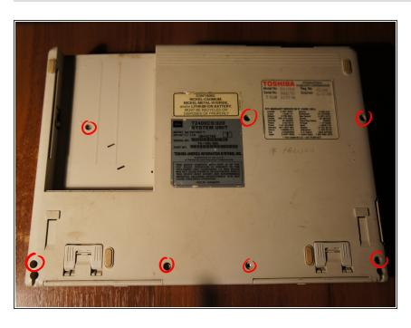
The bottom of the laptop has 6 visible screws and the 7th one is hidden under the battery
