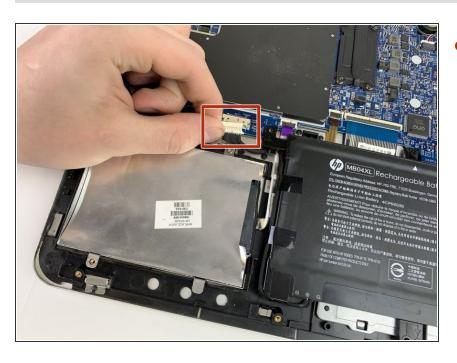
Disconnect the power supply cable connected to the motherboard.
