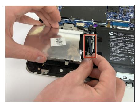
Disconnect the cable plugged into the hard drive and remove the hard drive from the device.
