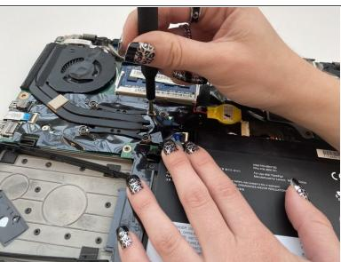
Use a Phillips #1 screwdriver bit and remove the four 3.0 mm screws from the heatsink.
