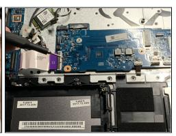
Remove the six 3.5mm screws that secure the motherboard to the laptop using a Phillips #00 screwdriver (PH00 bit).
