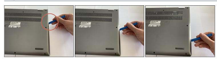
• Use a plastic opening tool to gently pry open the back cover.
