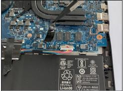
• Using tweezers, remove the piece of black tape over the battery cable connector.
