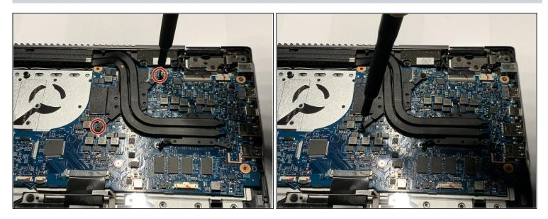
Remove the two 3.5mm screws that secure the heatsink using a Phillips #00 screwdriver (PH00 bit).
