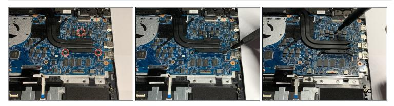
Remove the three 3.5mm screws that secure the heatsink using a Phillips #00 screwdriver (PH00 bit).
