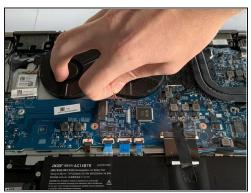
Grip the cord that connects the fan to the motherboard and gently pull out to disconnect the cable from the connector.
