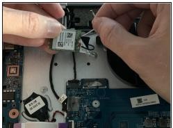
• Using your fingers, carefully pull the white wire upwards, removing it from the terminal of the wireless card.
