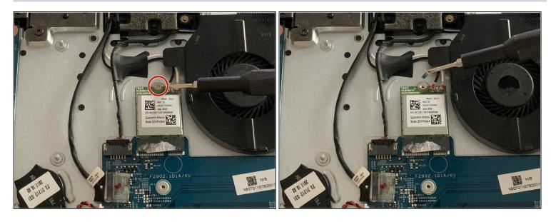
Remove the 6.5 mm screw that secures the wireless card using a Phillips #00 screwdriver (PH00 bit).
