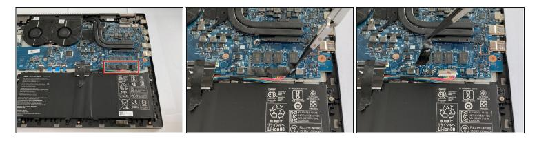
Using tweezers, remove the piece of black tape over the battery cable connector.
