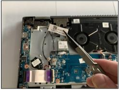
Using tweezers, remove the sticker that covers the connection between the wireless card and motherboard.
