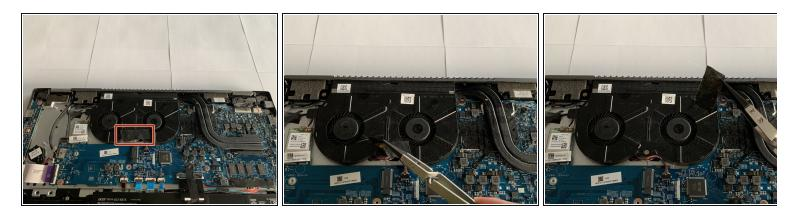
• Remove the piece of tape covering the fan screw using a pair of tweezers.
