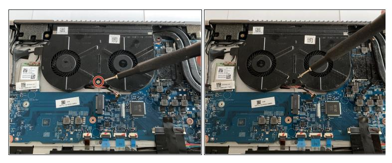
Remove the 3.5 mm screw connecting the fan to the computer using a Phillips #00 screwdriver (PH00 bit).
