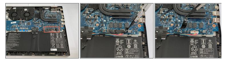
• Using tweezers, remove the piece of black tape over the battery cable connector.
