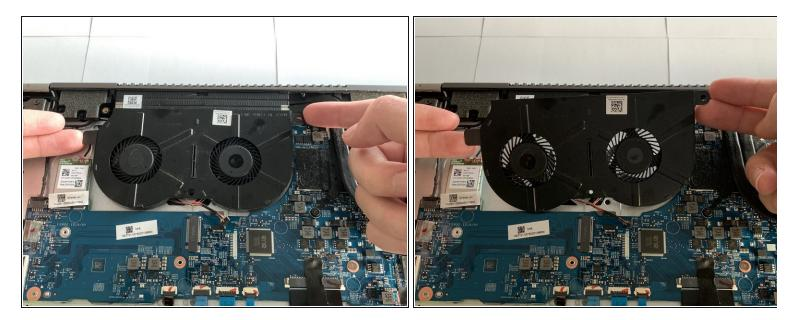
• Grip the fan with your fingers by the edges and lift up to remove the fan.
