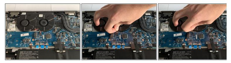
• Grip the cord that connects the fan to the motherboard and gently pull out to disconnect the cable from the connector.
