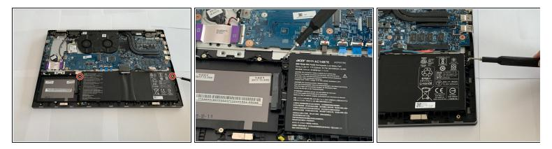
Remove the two 3.5 mm screws that secure the battery using a Phillips #00 screwdriver (PH00 bit).
