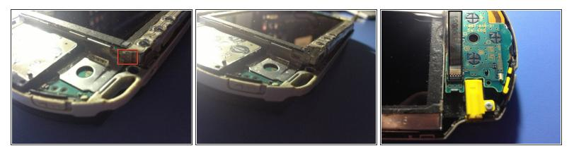
• This is one of the two clips which the button board has. With an oppener tool you should release it.
