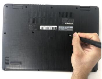
• Use a Phillips #1 screwdriver to remove the thirteen 6.5mm screws that secure the back cover.
