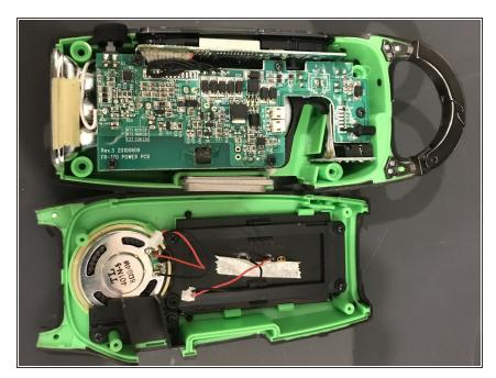
After pulling away the cables from the 2 plugs, we are free to keep tearing down!
