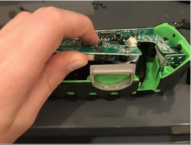
• There are 5 Phillips head screws securing the power board in place. Removing them allows some give to peek inside.
