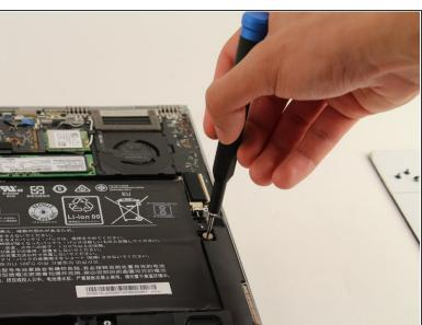
Remove the four silver 3mm JIS #00 screws holding the speakers in place.
