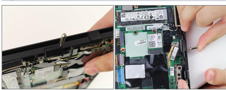
• Using an iFixit SIM card screw head tip, apply pressure to the hole to disconnect the SD card slot from the device.
