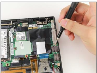
Use a Phillips #00 screwdriver to remove the two 3mm screws that secure the IO bracket.
