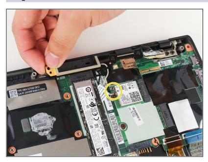
Lift the white and black wires from their press on connections. Make sure to grab the connector head, not the wire itself
