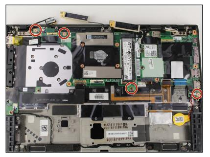
Use a Phillips #00 screwdriver to remove each of the four remaining 3mm screws securing the motherboard to the device.
