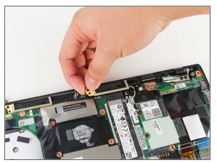
Lift from the location of the screw towards you. Then pull towards the screw side to remove the bracket.
