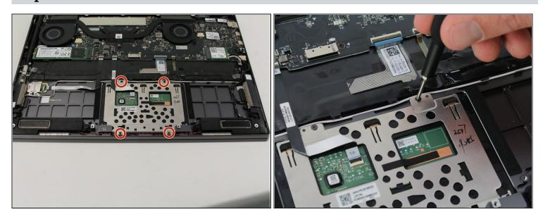
Unscrew the four 2 mm screws with a Phillips #00 screwdriver.
