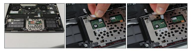
• Carefully pull out the small electrical wire from the back of the touch pad.
