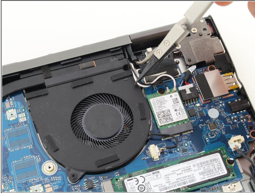
**i** When the laptop is upside down, the left fan is on the right side of the laptop near the wireless card and the SSD.
