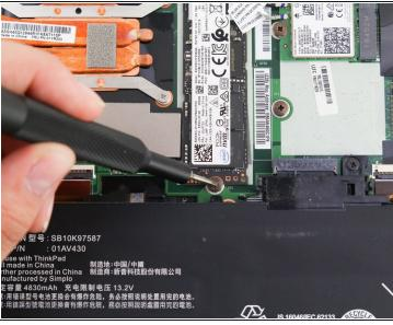
Use a Phillips #0 screwdriver to remove the single screw that secures the SSD to the motherboard.
