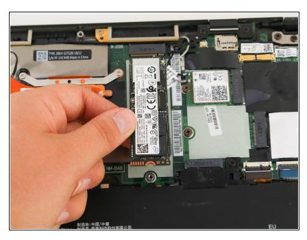
Carefully remove the SSD by lifting it and pulling it out of the pins towards the battery of the laptop.
