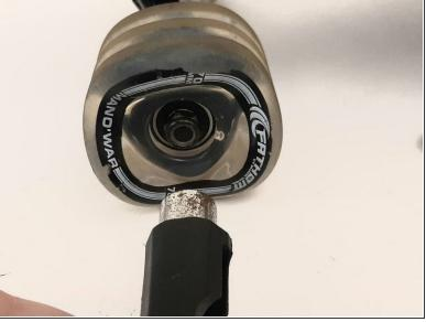
• Using the 1/2" side of the Skate Tool, screw the nut back on the axle to hold the wheel in place.
