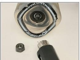
• On a flat surface, unscrew the nut that holds the wheel on the axle using the correct size from the skateboard tool (1/2" size, typically the smaller of the 2 on the top of the 'T') and turning to the left.
