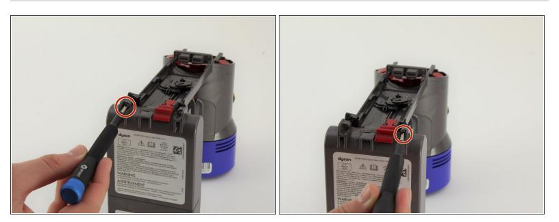
• Use a Phillips #0 screwdriver to remove two 18 mm screws on the bottom of the battery.
