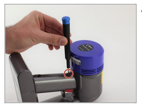
Use a Phillips #0 screwdriver to remove one 18 mm screw on the back of the handle.
