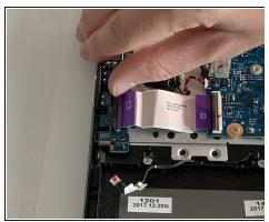
Place your fingernail underneath the locking black tab of the ZIF connector on the USB/Side
