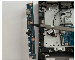
• Using tweezers, gently grip the middle of the board that contains the side ports and carefully pull out to remove it.
