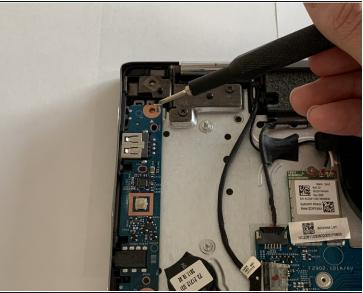
Remove the two 3.5mm screws that secure the side ports using a Phillips #00 screwdriver (PH00 bit).
