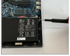
Remove the two 3.5 mm screws that secure the battery using a Phillips #00 screwdriver (PH00 bit).
