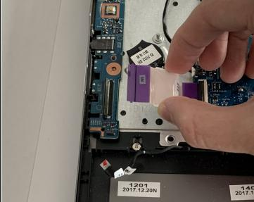
• Remove the ribbon interconnect cable from the connector.
