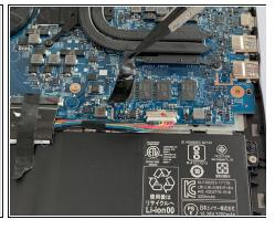
• Using tweezers, remove the piece of black tape over the battery cable connector.
