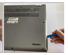
• Use a plastic opening tool to gently pry open the back cover.
