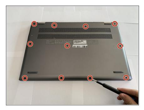
Remove the eleven 6.5 mm screws that secure the back case using a Phillips #1 screwdriver.
