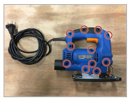
Close and screw the device back together.
