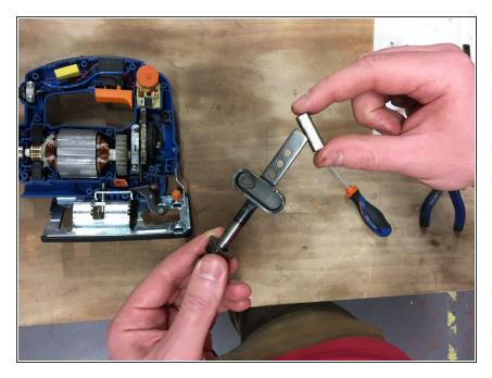
First, put the slide onto the new blade bracket.
