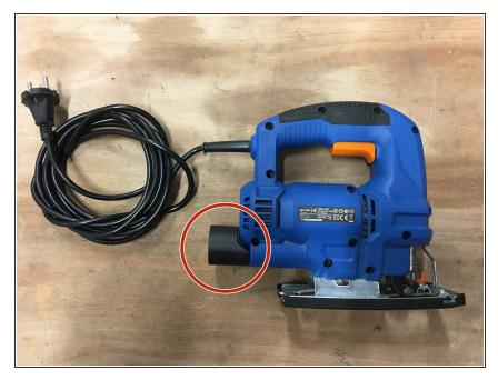
Remove the vacuum hose adapter at the back of the device.
