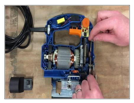
Take off the blade holder, then raise the slide located at the end of the holder.
