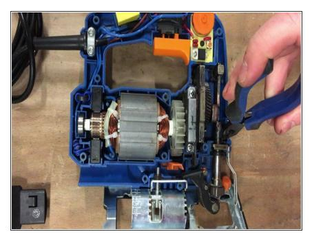
Using pliers, remove the clip beside the blade holder.
