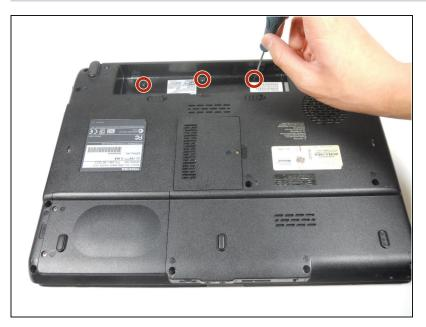
• Remove the three 3.7 mm type-00 Phillips head screws located in the battery compartment, per image 1.
