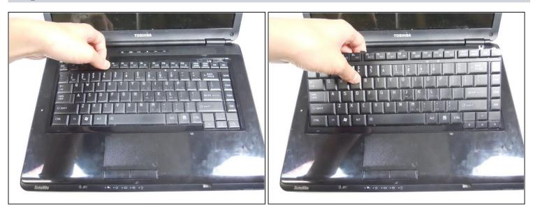
• Starting at the top, gently raise the keyboard enough to remove it from the socket.
