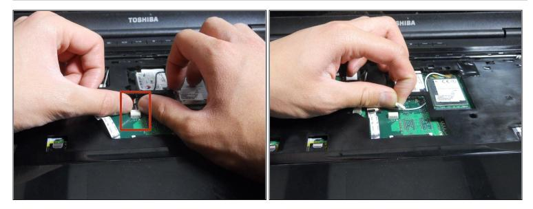
• Using your fingers, remove the white plastic connector located to the right of the ribbon connector, per image 1.
