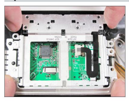
Using your fingers, remove the metal framing surrounding the touch pad by pulling upwards on each of the four corners.
