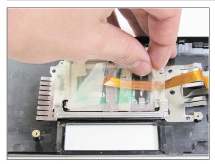
Using your fingers, remove the plastic film that covers the two connectors to the touchpad.
