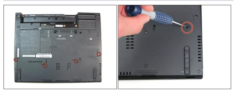
Using a #0 Phillips screwdriver, remove the four 17.0 mm screws.
