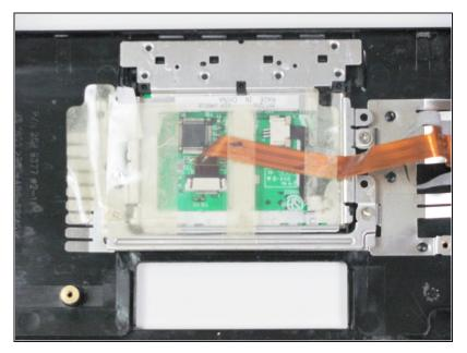
Turn the palm rest over to access the back of the touch pad.
