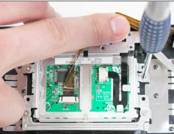
• Use a #0 Phillips screwdriver to unscrew the four 3.4 mm screws circled in red.
