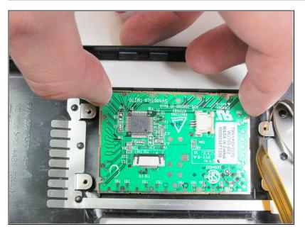
Remove the touch pad by lifting it out of the palm rest with your fingers.
