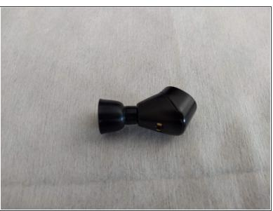
Let's start by the basics, take the earbud(s) out and remove the silicone tip by pulling the cup outwards
