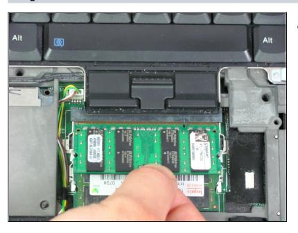
Remove the memory card from the slot by pulling perpendicular to the slot.
