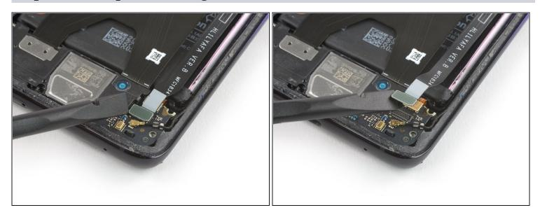
• Use a Spudger to pry up and disconnect the interconnect flex cable from the daughterboard.
