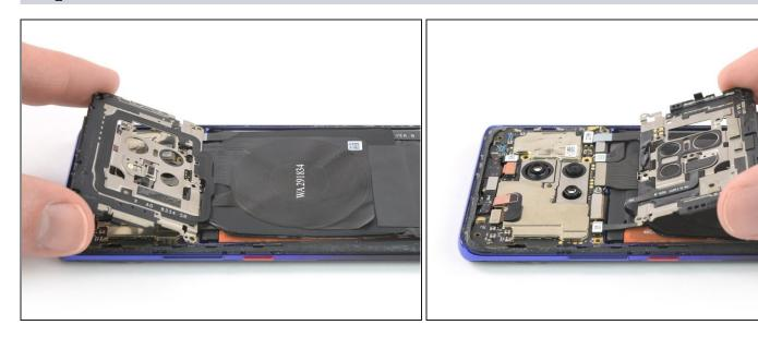
• Carefully fold the motherboard cover in the direction of the battery.
