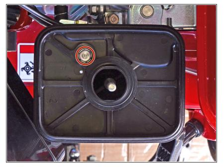
Use a 10 mm socket and socket wrench to remove the 25.5 mm-long bolt securing the air filter elbow to the tiller.
