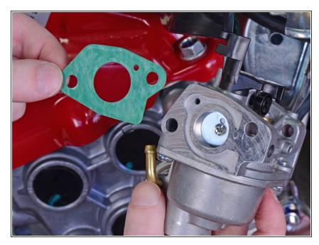
(i) The outlet on the rear of the carburetor has a thin gasket. Inspect the gasket's condition and replace if needed.
