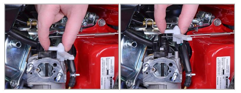
Pull the choke lever straight up to remove it from the carburetor.
