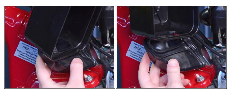
Hold onto the air filter hose and pull on the air filter cover to remove it.
