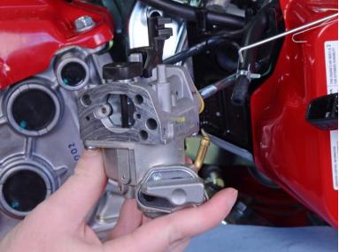
Pull the carburetor straight off of the threaded rods to remove it.
