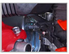
Use a pair of snap ring pliers to loosen the spring hose clamp on the breather tube, pulling it out 2-3 cm so it's not clamping onto the end of the tube.
