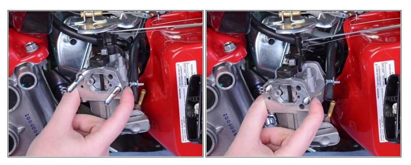
Pull the carburetor halfway out, but do not completely remove it yet.
