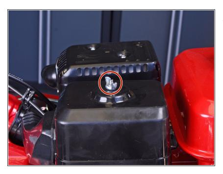
Use your fingers to unscrew and remove the wing nut securing the air filter cover to the air filter elbow.
