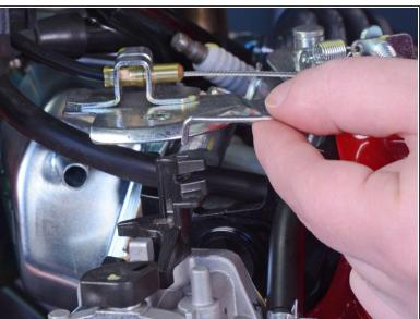
Grab the governor rod and lift it straight up to remove it from the carburetor.
