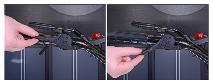
• Push the throttle lever all the way down.
