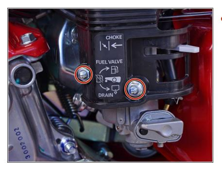
Use a 10 mm socket and socket wrench to remove the two nuts securing the air filter elbow to the carburetor's threaded rods.
