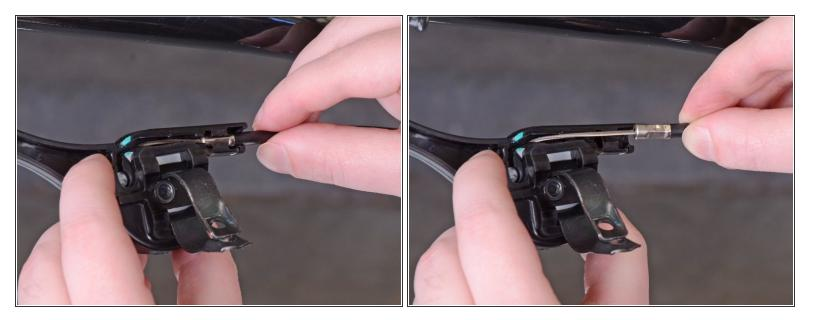
• Grab the open end of the throttle cable and pull it out of the throttle lever to free it from its recess.
