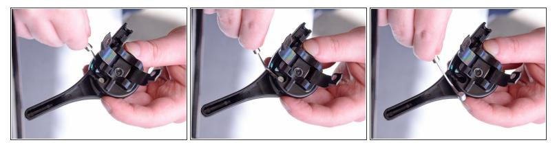
Continue to lift the throttle cable out of the throttle lever, making sure it clears the openings in the recess.
