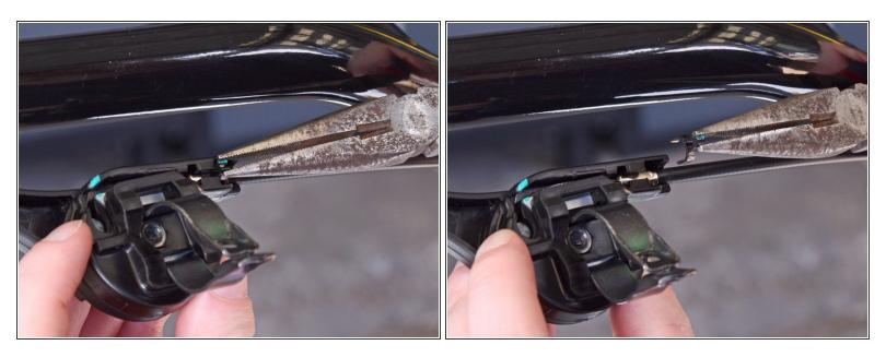
• Use a pair of needle-nose pliers to remove the small clip attached to the throttle cable.
