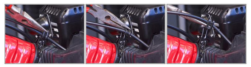
Use a pair of needle nose pliers to bend the metal clip at the bottom of the handle column out and upward.
