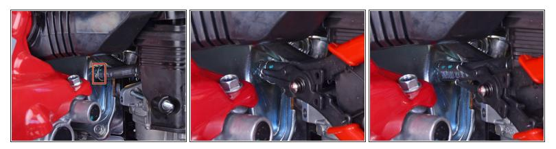
Use a pair of snap ring pliers to loosen the spring hose clamp on the breather tube, pulling it out 2-3 cm so it's not clamping onto the end of the tube.
