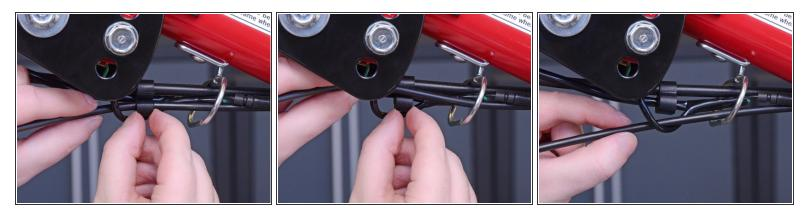
• Pull the throttle cable out of the cable holder underneath the handle column.
