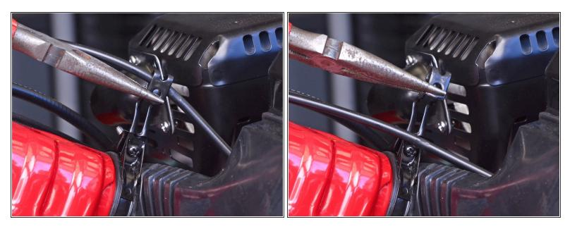
• Use a pair of needle nose pliers to bend the last section of the metal clip outward to release the throttle cable.
