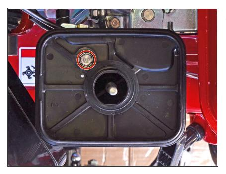
Use a 10 mm socket and socket wrench to remove the 25.5 mm-long bolt securing the air filter elbow to the tiller.
