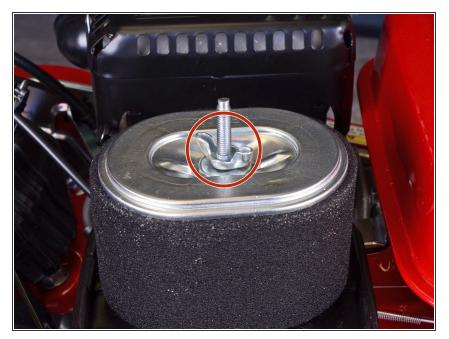
Use your fingers to unscrew and remove the wing nut securing the air filter to the air filter elbow.
