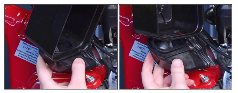
• Hold onto the air filter hose and pull on the air filter cover to remove it.
