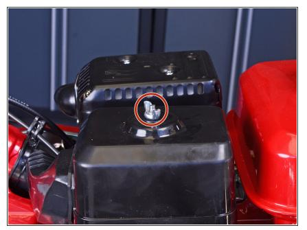
Use your fingers to unscrew and remove the wing nut securing the air filter cover to the air filter elbow.
