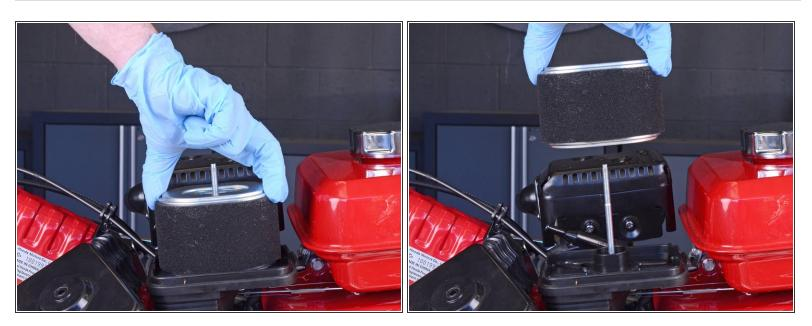
(i) Wear gloves or use a rag during this step, as the air filter is coated with oil.
