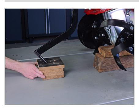
Place a block (or blocks) of wood under the tiller's drag bar to prevent the tiller from leaning back.
