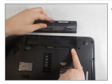
Hold the left notch in an unlocked position with one hand and use the other hand to slide the battery out.
