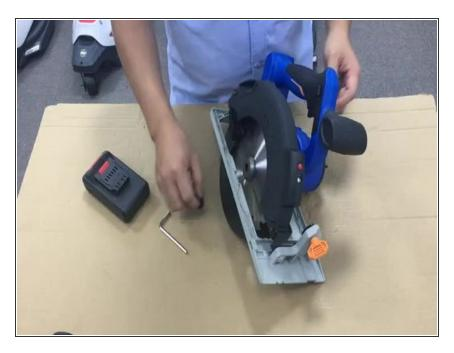
Remove the blade and the internal flange.
