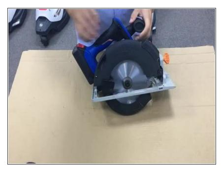
Remove the battery from the <u>circular</u> <u>saw</u>. Turn the Allen wrench to detach the external flange.
