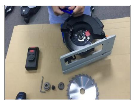
Remove the tension spring. Remove the screw of the bottom guard.
