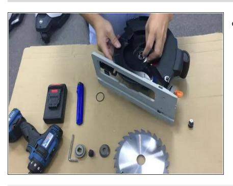
Remove the bottom guard from the device.
