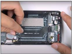
• Use your fingers to remove the LED flex cable, CED flex cable, and USB port cable.
