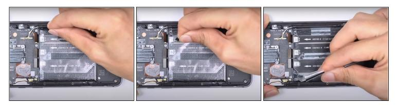
• Use your fingers to grab the black tab and remove the plastic that was underneath the battery.
