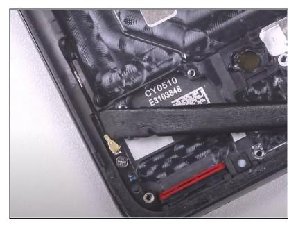
Disconnect the coaxial cable in the lower left-hand corner using the flat end of a spudger.
