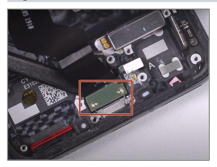
Use the flat end of a spudger to disconnect the USB port flex cable.
