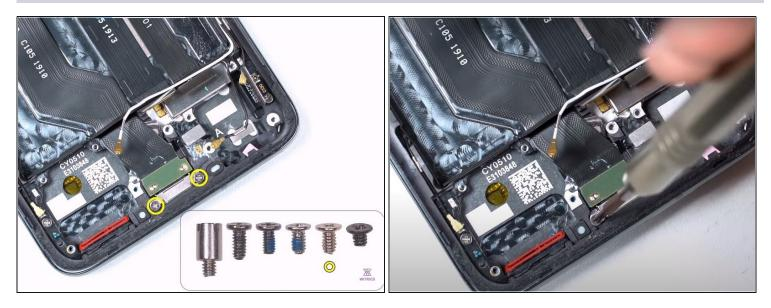
Use a Phillips #000 screwdriver to remove two screws.
