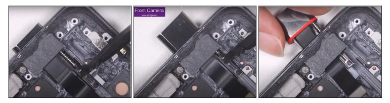
• Use the flat end of a spudger or your fingers to gently remove the front camera assembly.
