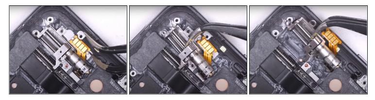
• Use a pair of tweezers to remove the camera elevator assembly.
