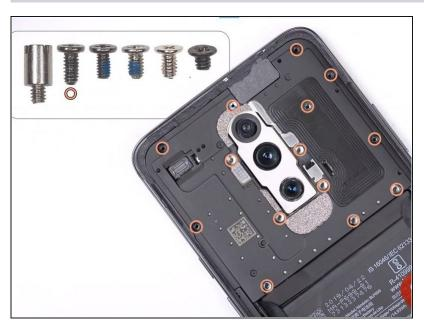
Use a Phillips #000 screwdriver to remove the fourteen screws from the plastic motherboard cover.
