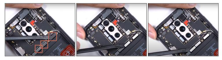
• Use the flat end of a spudger to disconnect the display and touch flex cable, main flex cable, and USB port cable.
