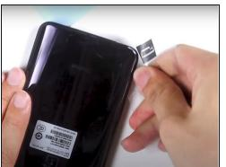
• Use a plastic card or Jimmy tool to slice around the phone's seam, cutting through the adhesive.
