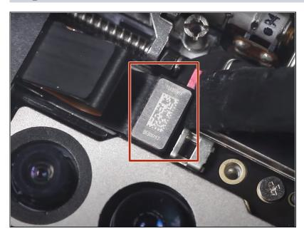
Use the flat end of a spudger to disconnect the connector that was underneath the red plastic tab.
