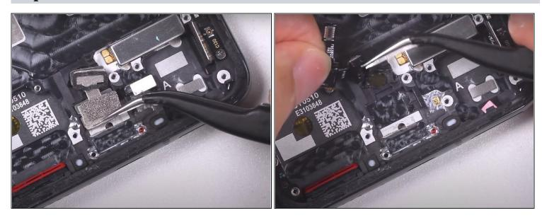
• Use a pair of tweezers to disconnect the fingerprint sensor.
