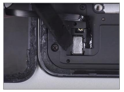
Use the flat end of a spudger to disconnect the laser autofocus and flash flex cable.
