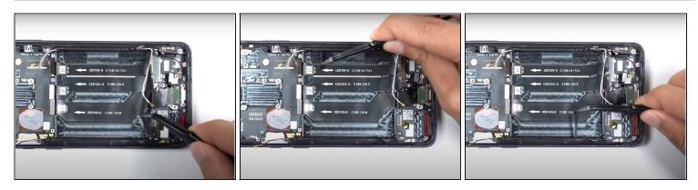
• Use a pair of tweezers to peel out the black stickers from the sides and bottom of the battery area.
