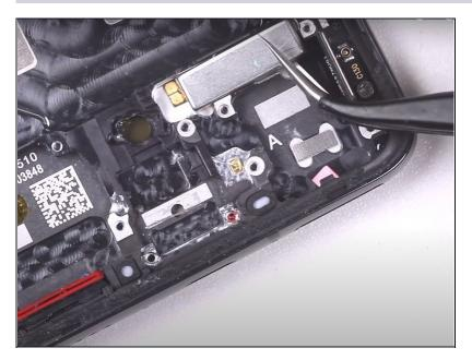
Remove the vibration sensor using a pair of tweezers.
