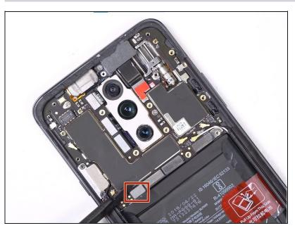
Use the flat end of a spudger to disconnect the power flex cable.
