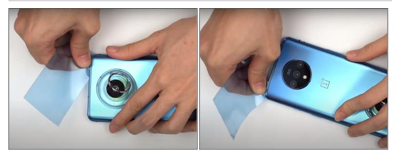
• Use a plastic card or Jimmy tool to slice around the phone's seam, cutting through the adhesive.
