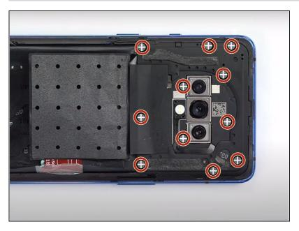
Use a Phillips screwdriver to remove the 11 screws from the plastic motherboard cover.
