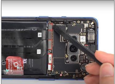
• Use the flat end of a spudger to disconnect all flex cables leading to the motherboard.
