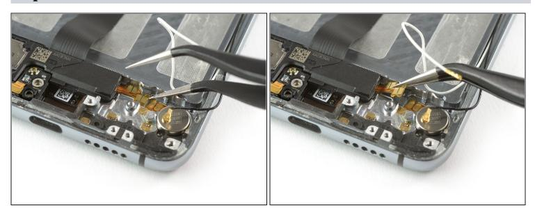
• Use one arm of a pair of <u>tweezers</u> to peel up the contact cable of the loudspeaker.
