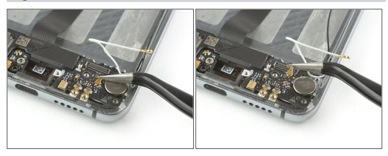
• Use a pair of <u>tweezers</u> to disconnect the black coax cable and fold it out of your way.
