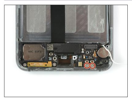
• Remove the two Phillips #00 screws (3.4 mm length).
