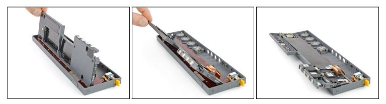
• Flip the midframe over to gain access to the flex cable connector underneath.
