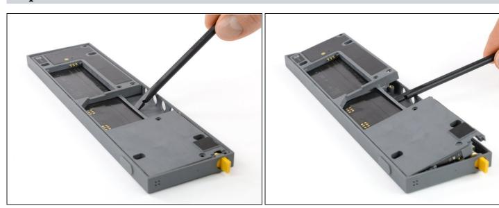
• Place a spudger in the cutout of the extension module to lift the midframe.
